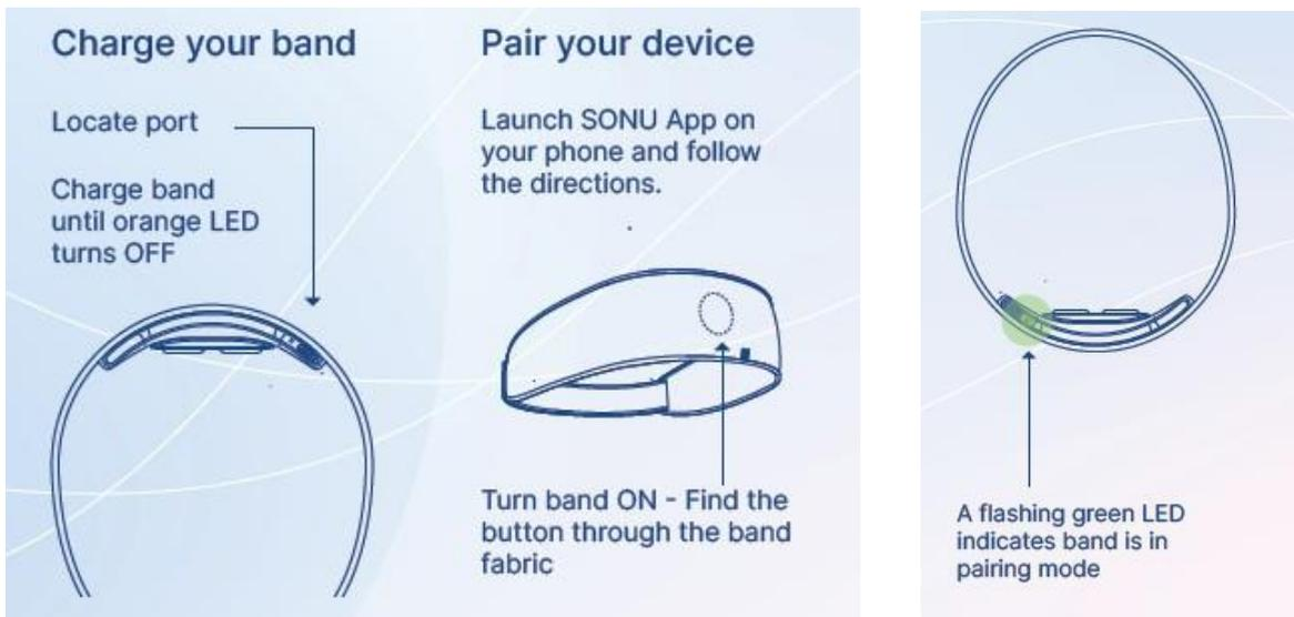
**Step 3:** Press and hold the power button until the Light Emitting Diode (LED) flashes green. This indicates band is in pairing mode and ready to connect to the iPhone via Bluetooth.
